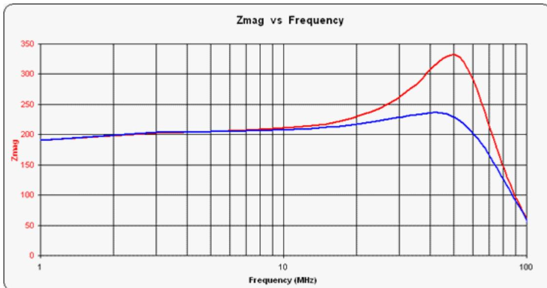
As before the red trace is without the compensation capacitor, the blue trace is with it fitted.
