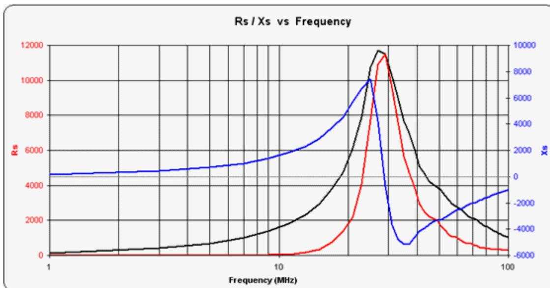
The next stage of the tests was to measure the input impedance of the Unun when the secondary was terminated in a 5K ohm load. The intention of this test was to simulate the performance of the Unun when presented with the sort of load impedance that was likely to be encountered when attached to a 1/2 wave antenna.
