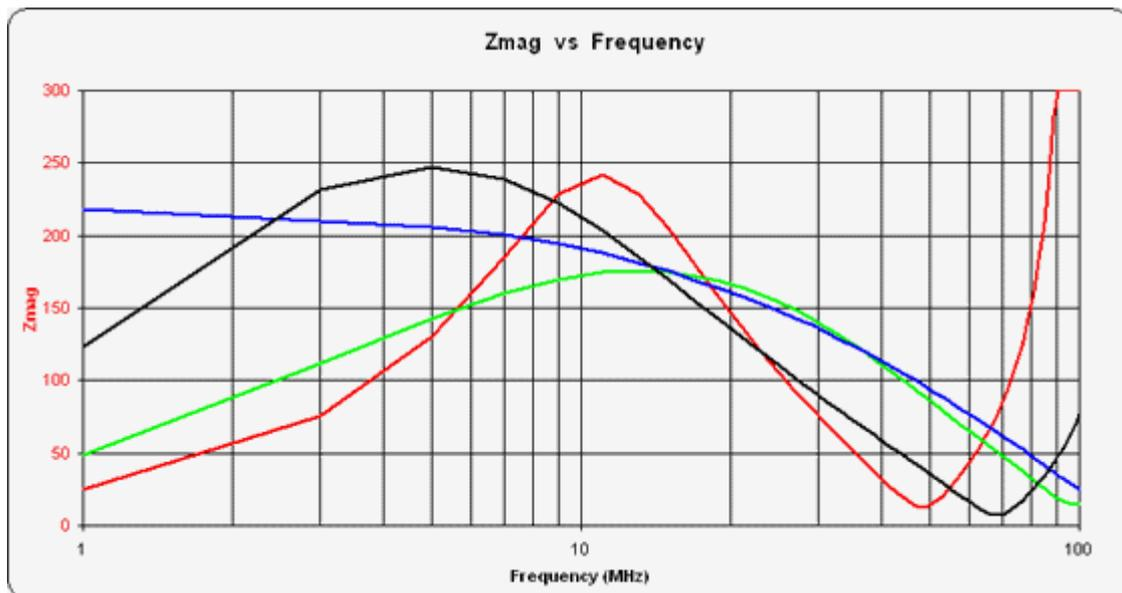
This time I have also measured the output when the input is terminated with 220 ohms. The target impedance is 880 ohms.
