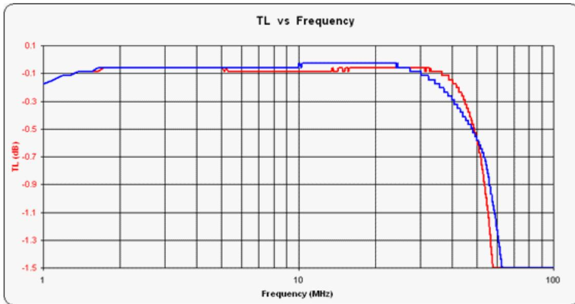
The red trace is without the compensation capacitor, the blue trace is with it fitted.
