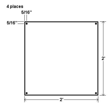
Form the box by screwing through the holes in the corners of a piece of
