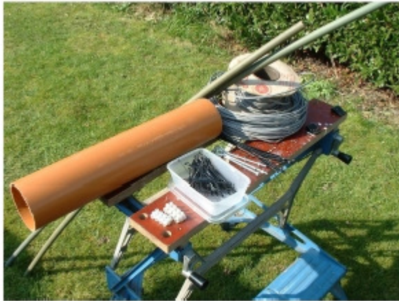
Materials 4inch tube, choc blocks, cable ties, hardware
