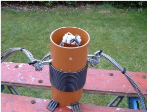
Ugly Balun showing aerial element connections
