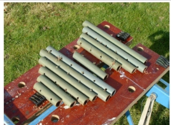
22mm PVC tube cat to size for both elements
