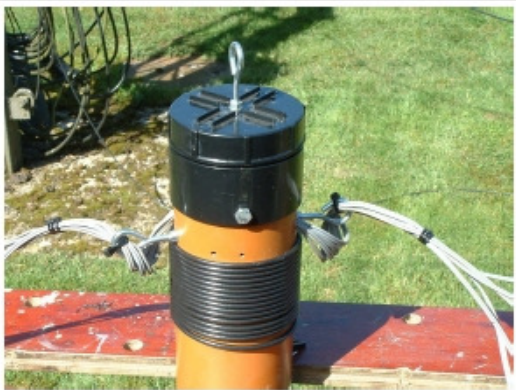
Completed Ugly Balun with connected dipoles
