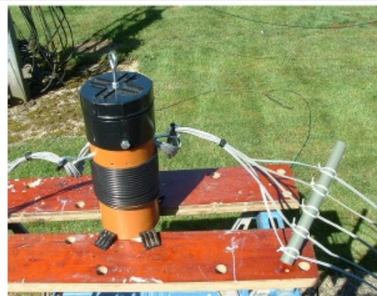
Completed Ugly Balun with connected dipoles Each element is cable tied to spacing insulator
