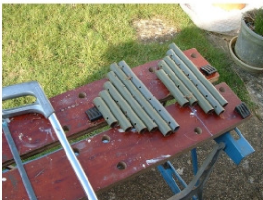
22mm PVC tube cat to size for both elements
