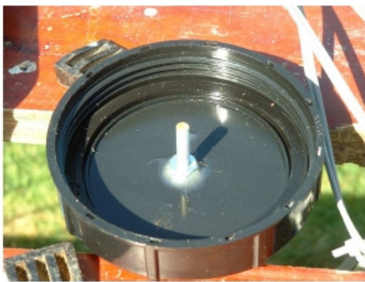
4 inch pipe cap with fixing nut glued in place with araldite.
