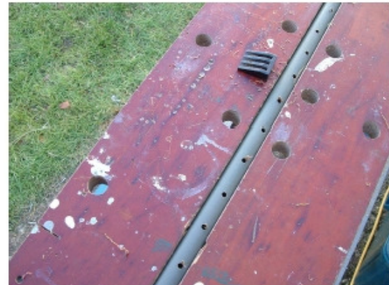
22mm 'PVC' tube drilled M5 holes 40mm apart
