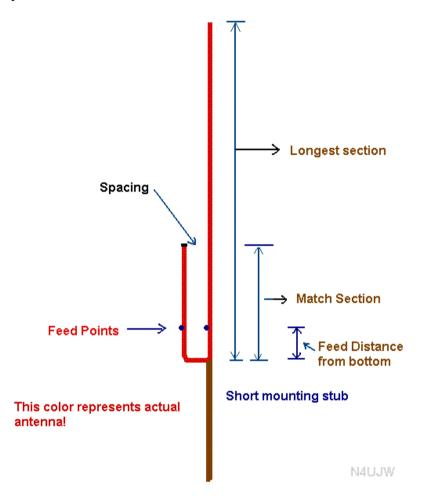
Note in the drawing above the wording, "This color represents the actual antenna!", refers to the red/orange color, not the brown color to the right of the wording. That is the support for the J pole.
