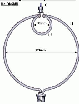
C = air- or vacume capacitor of 0...20pF L1 = 1/4 wave: for 145MHz use a copper or brass wire with a length of 49cm and at least 3mm in diameter.
