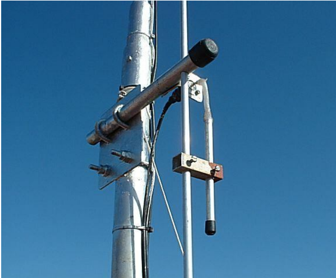
Photo: Showing the Gamma Match of the Dip-Yag Antenna
