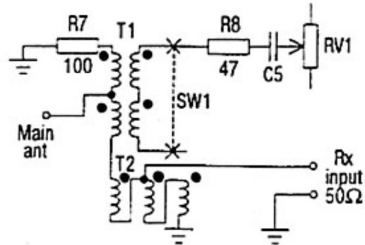
T2 - 8 turns tri-filar wound on an Amidon FT50-72 toroidal ferrite core
