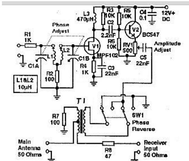
**Figure 2 Interference Cancelling Circuit**
