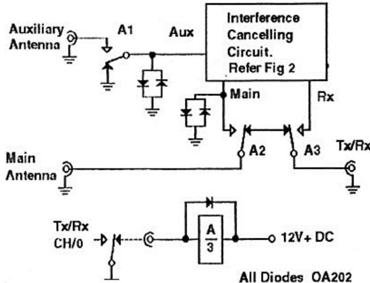
Figure 4 - Transmit-Receive Switching
