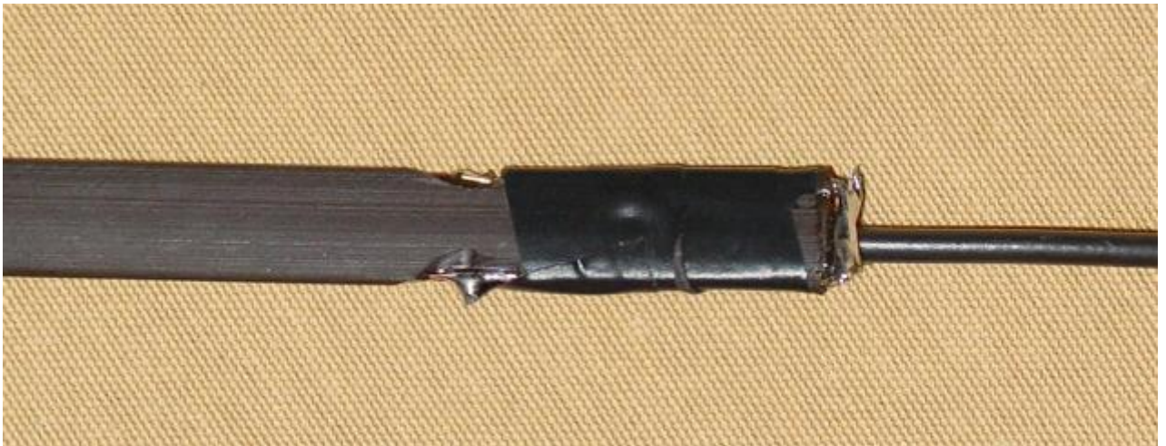
The same construction with 300-Ohm-wire. The cable is available at DX-Wire
