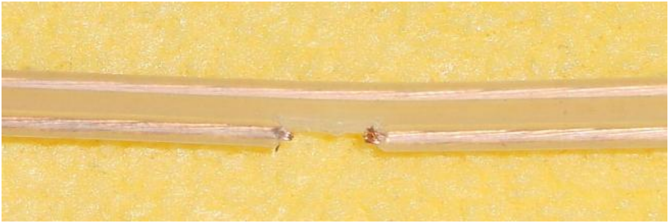
The cut piece of wire between the parts A and B at the right side of the J-Pole
