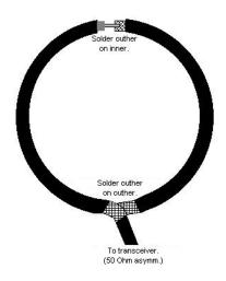
The coupling loop has a diameter of 15 cm and is made of RG58 coax. It's called a shielded- or Faraday loop. You can click on the image right of this text for the construction details. It is not connected to the main loop and should be placed opposite of the tuning capacitor. The loop is coupled directly to the transceiver, no antennatuner is needed.
