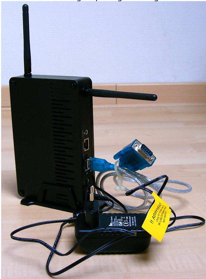
Figure 9. WiFi USB-2 Server and USB RS232 device used in WLAN network
