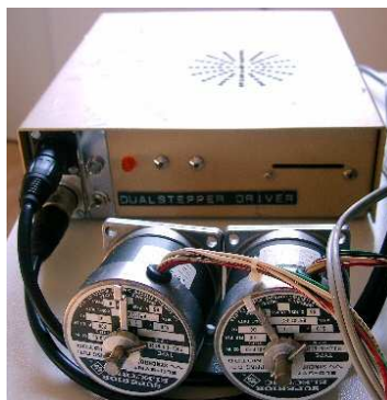
Figure 6. Housing for stepper circuits and in front of it two applied stepper motors
