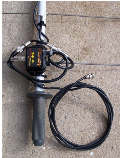
Photo n°4: Details of the elements fixed to the boom and feed line connected to the radiator.
