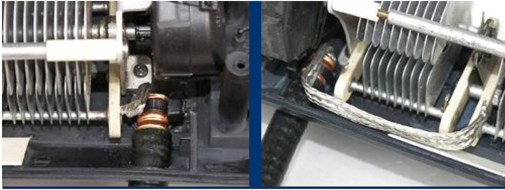
Variable capacitor soldering joints made with RG213 coaxial braid.
