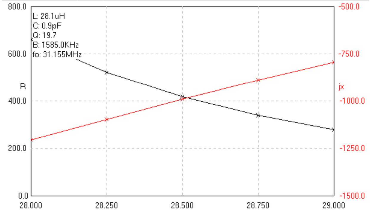
Antenna W3DZZ has input impedance close to 60 Ohms at 80 and 75 at 40, , so, a 75-Ohms coaxial cable can be used for feeding of the antenna.
