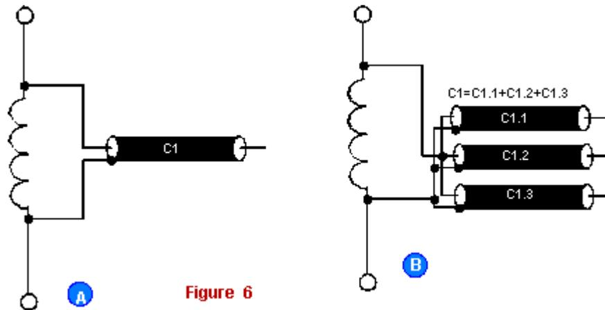
**Figure 6** A coaxial cable capacitor
