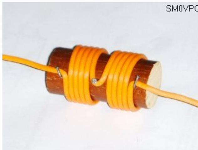
*The support nails for the coil, and the coil added.*
