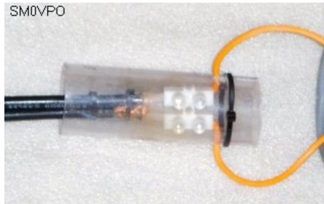
*The connector feeding the antenna elements.*
