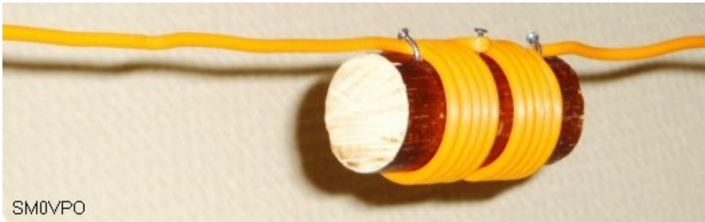
*The finished stub positioned in the antenna wire.*
