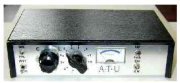
This Antenna Tuning Unit also incorporates a 50ohm QRP dummy load, power meter (1 or 10 Watts full scale), and SWR
