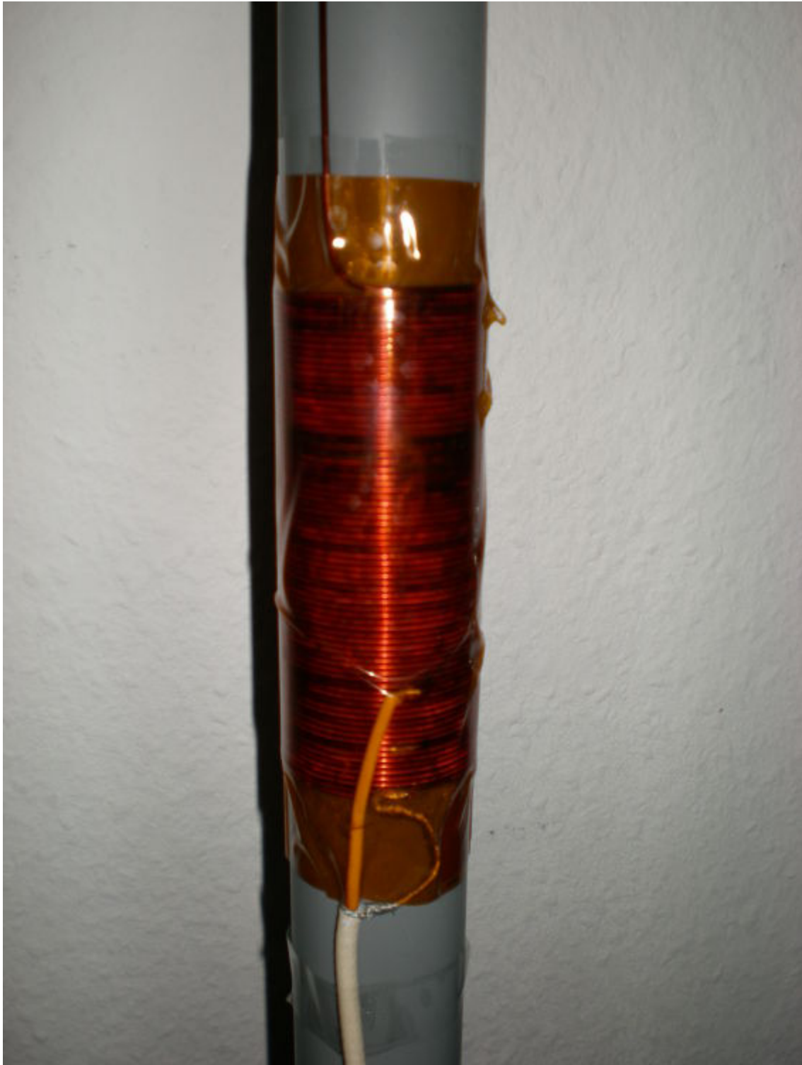
Here is a photo of the installed 80m antenna:
