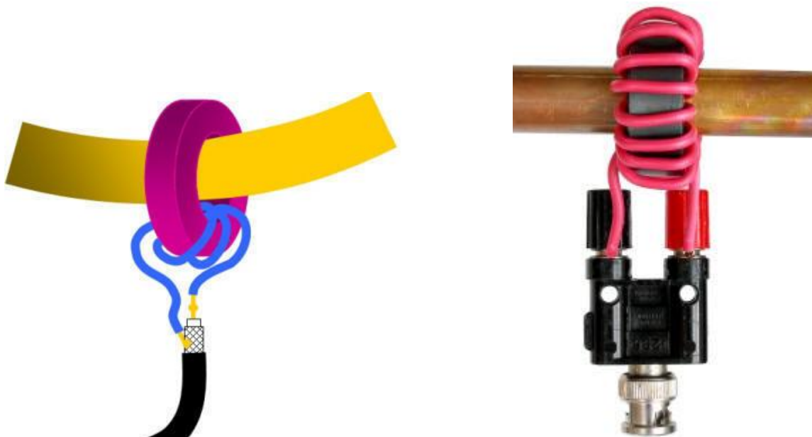
Coupling with a ferrite core toroidal transformer - multiple secondary windings
