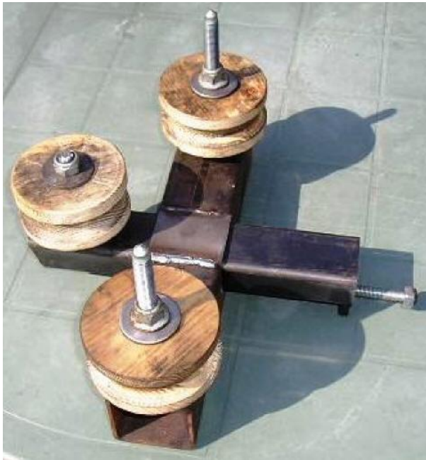
Tube roller made by Twan, PA0KV (photos used with permission)
