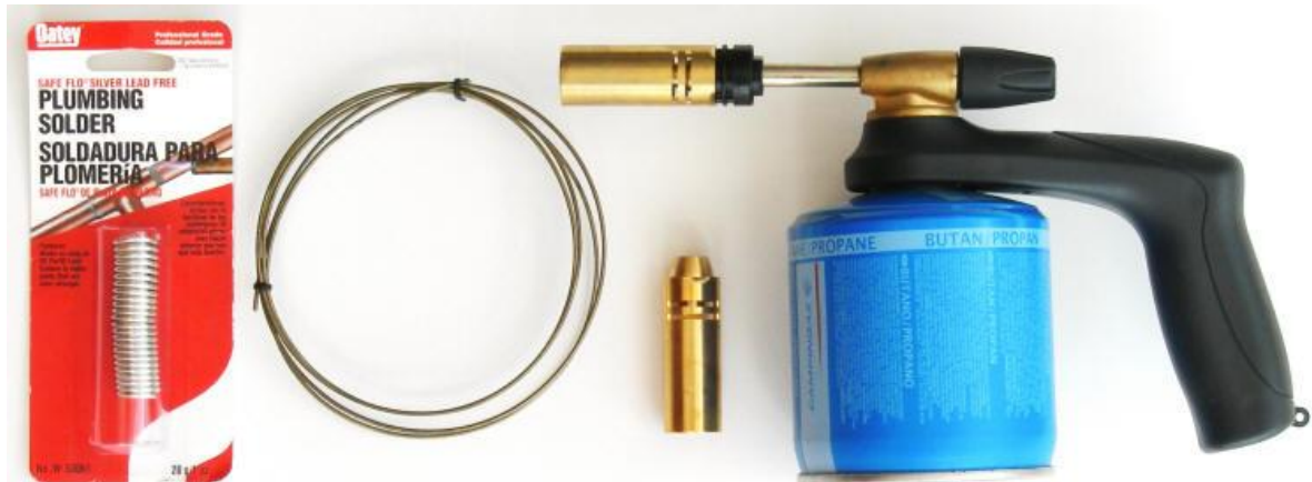
Soldering tools: blowtorch, two kinds of silver solder (flux not shown)
