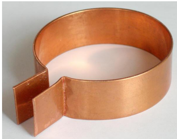
Capacitor clamp/bracket - made of a strip of 1x20 mm soft copper
