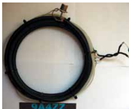
Slika 6. Collins balun 1:1, RG 213 namotan u smotuljak
