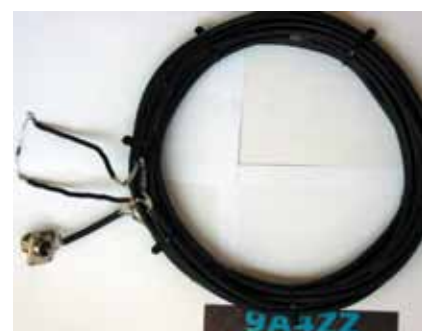
Slika 8. Collins balun 1:4, RG 58 C/U namotan u smotuljak
