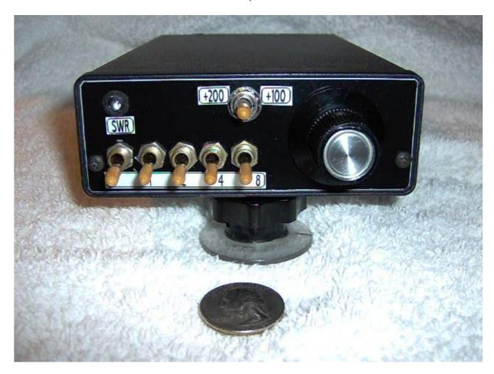
Since I got my Icom 703, I wanted a tuner to handle the 10 watts the 703 was capable of, and was designed to tune half wave endfed wires which is one of my favorite field antennas. I also wanted it to cover at least 10 thru 80 meters, thus the Switched Inductor L Match Tuner was born.
