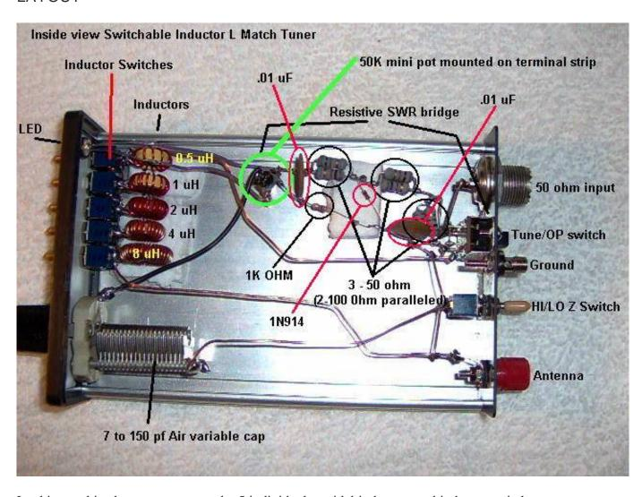
Looking at this photo, you can see the 5 individual toroidal inductors and inductor switches
