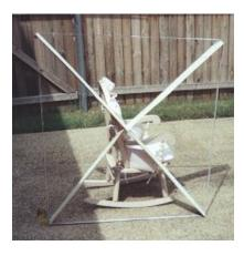
The three foot ribbon cable loop assembled, propped up by a child's rocking chair - it is not self supporting. This is a very "hot" design - excellent "Q" and excellent sensitivity.
