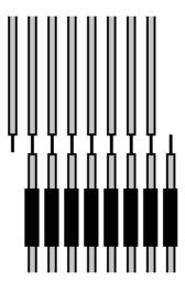
Connect conductor 1 of the ribbon cable to the ground terminal of the tuning capacitor, the other end of the other side to the other terminal of the tuning capacitor.
