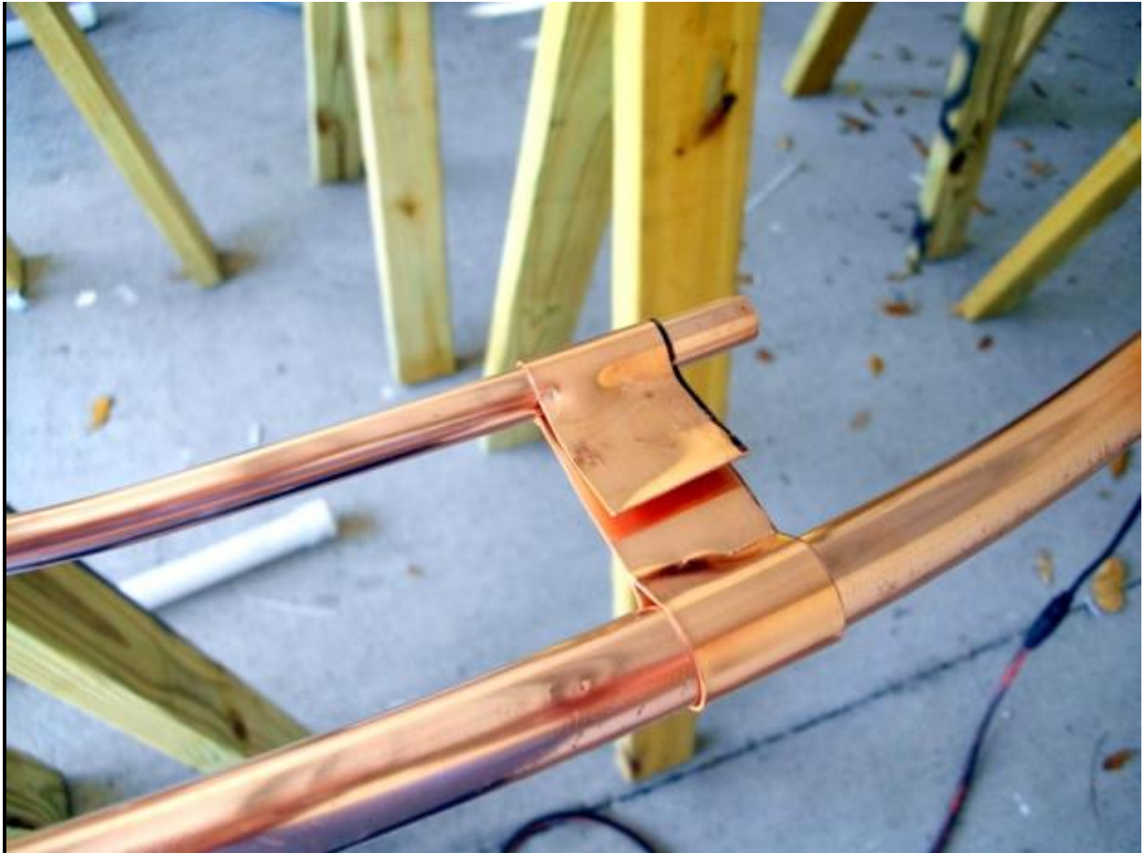
Making the clamp for the Gamma Match
