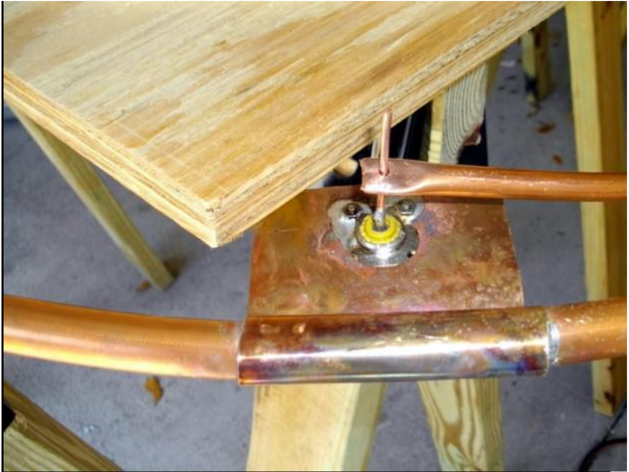
Soldering The Back Plate and PL 259
