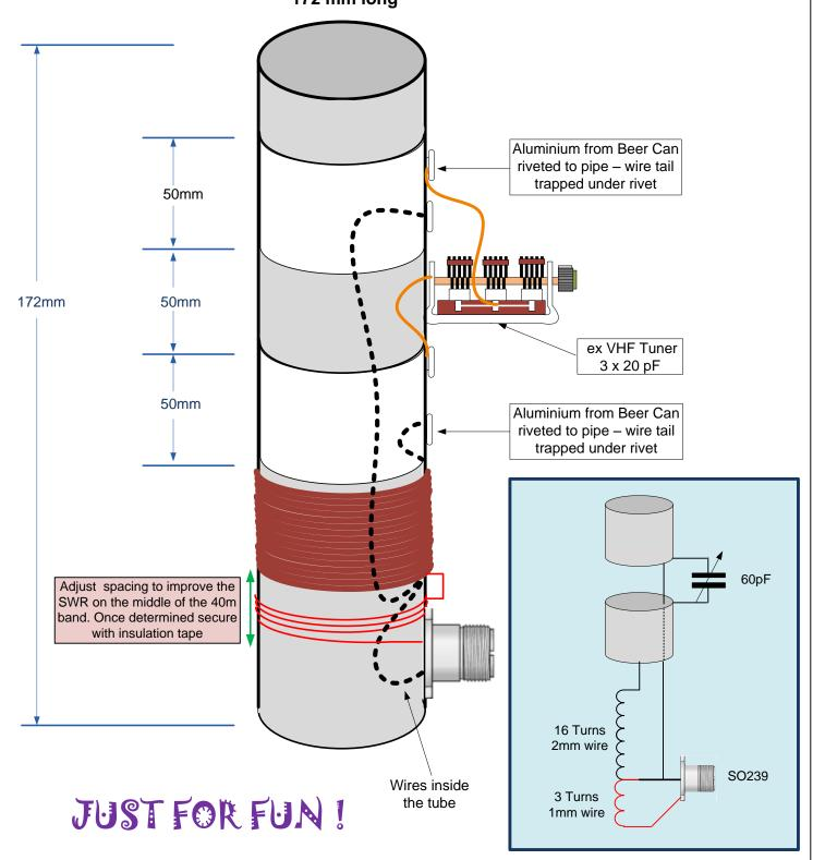
The two aluminium 50 mm tubes form a capacitor, and together with the variable capacitor are wired in parallel with the 16 turns coil. The antenna is coupled with the second coil of 3.5 turns coil. that connects the SO239 socket directly feeding the radio. The Tuning is sharp and the antenna exhibits a bandwidth of about 80KHz (SWR 2:1)
