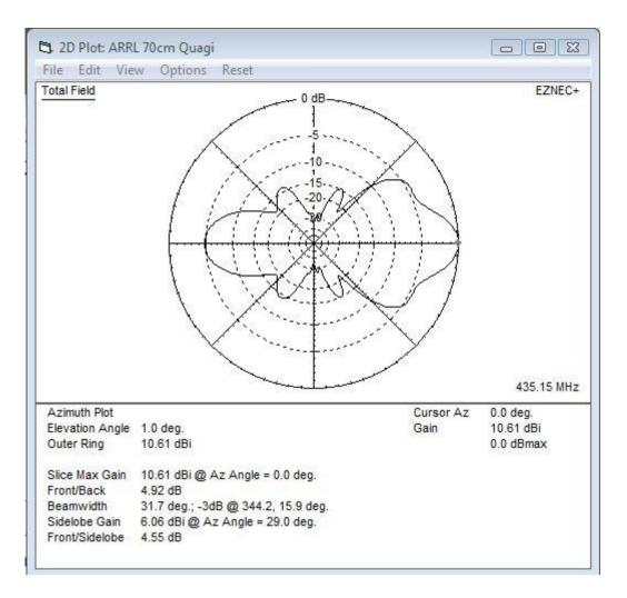
In this graph we are looking down onto the antenna with the directors in the horizontal position. The reflector and driven element quads are to the left. The directors run off to the right. The highest gain is to the right, in the direction of the directors, at 10.61 dBi.
