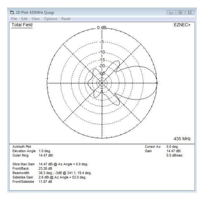
The antenna has gone from a ho-hum performer to one with some serious specs. First off the front-to-back ratio now rivals the kind of rejection (25 dB) talked about in the literature. Its front-to-back ratio of 23.26 dB is quite good. Second, the gain of 14.47 dBi is as good as some Uda-Yagi antennas of twice the number of directors.
