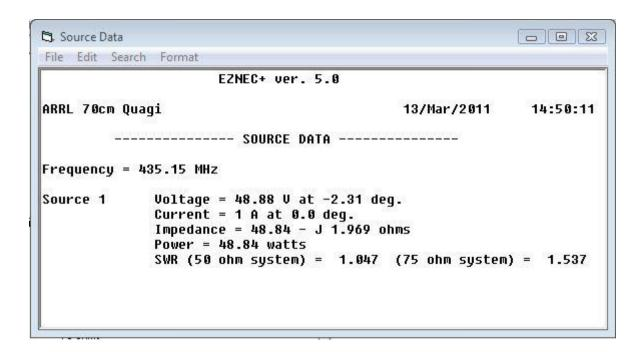
This is a pretty good match to  $50 \Omega$  coaxial cable but the gain is modest and the front-to-back ratio is pretty low.
