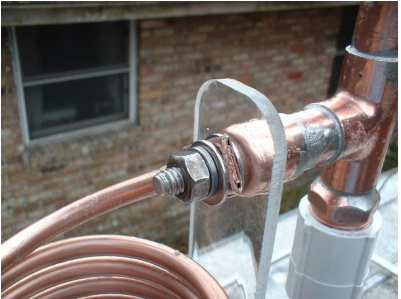
This is a close-up picture of one of the ends of the loading coil.
