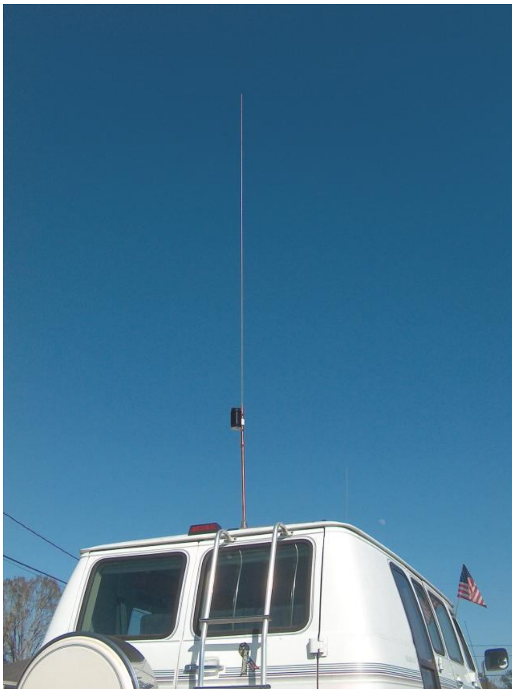
The 40 meter loading coil installed on the antenna.
