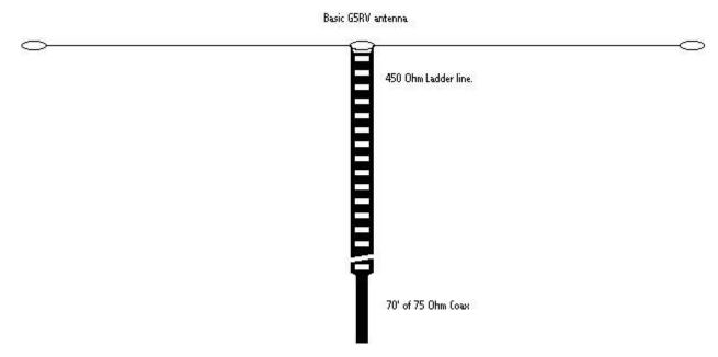
So, to figure a conventional G5RV, we devide 1428 by 14 Mhz, which equals 102 feet. This is the total length of the flat top section, and since it is fed at the
