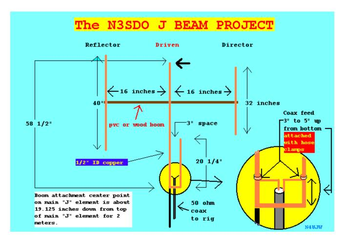
Notes: Make driven element about 2 feet longer at bottom for mast mounting.
