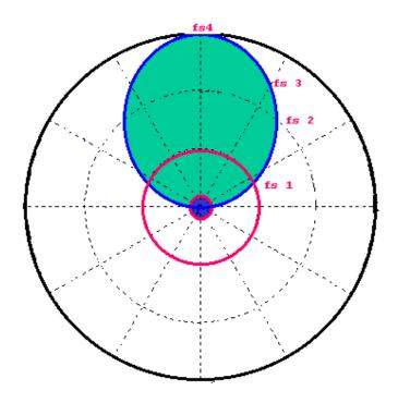
Red circle is pattern of standard omni J Pole Green area is estimated pattern of JBEAM using field strength meter readings
