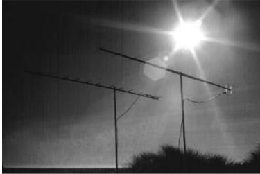
One answer is to measure the antenna's gain against a known reference. Antenna gain measuring sessions have been conducted at VHF/UHF conferences since the 1950s. Often these sessions, in which antennas are sometimes measured side by side as shown in the 1977 photo at left, are conducted by antenna experts using professional quality signal sources and measuring
