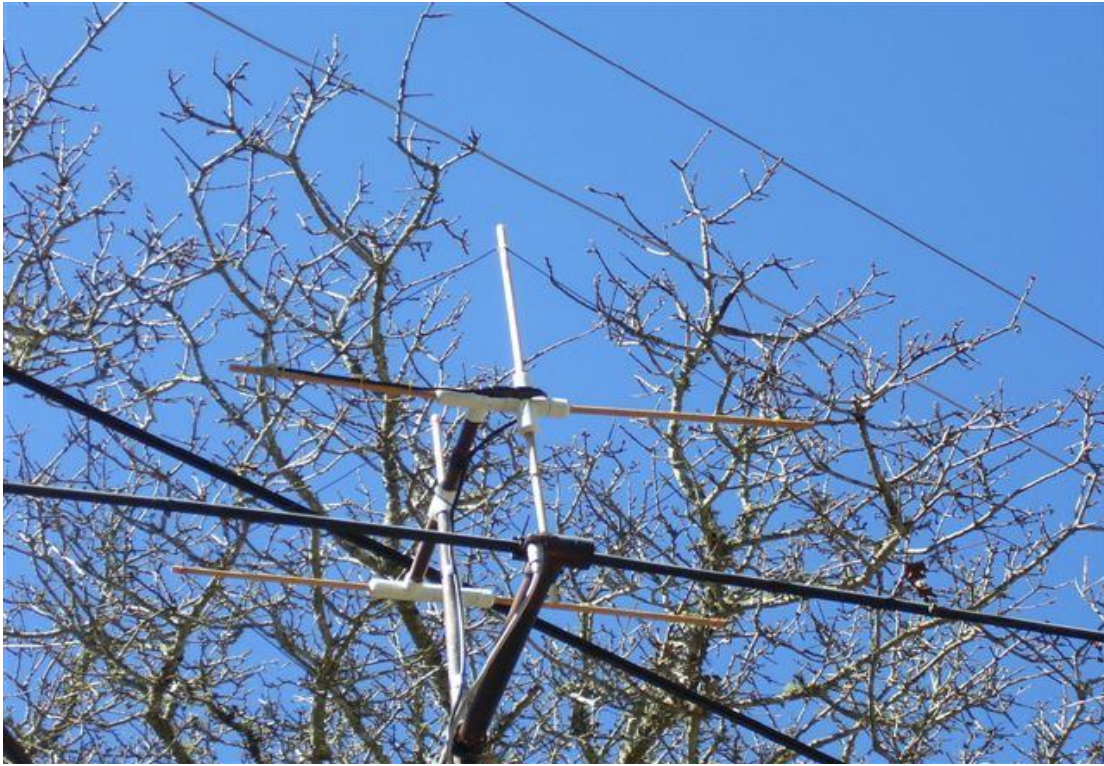
2 Meter 2 Element Quad shown mounted above another antenna with coax feed nearest you on left spreader rod.
