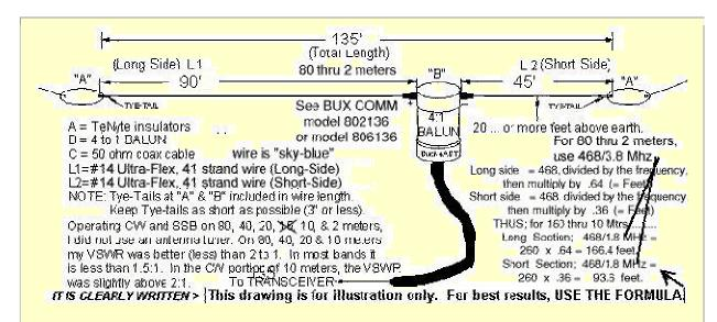
Similar to WINDOMs shown above, These WINDOMs are completely assembled, ready to connect the coax, and erect. BUXCOMM Windoms are power rated at 1000 watts SSB and include all insulators, high-tensile strength, super flexible PVC covering, Power-Flex, tinned, copper wire, connectors, and BALUN. Our High-power versions are rated at 2000 watts and are identified with an "HP" in the model number. See coaxial cable and related items below. You can be on the air in no time, with any of our Windoms.
