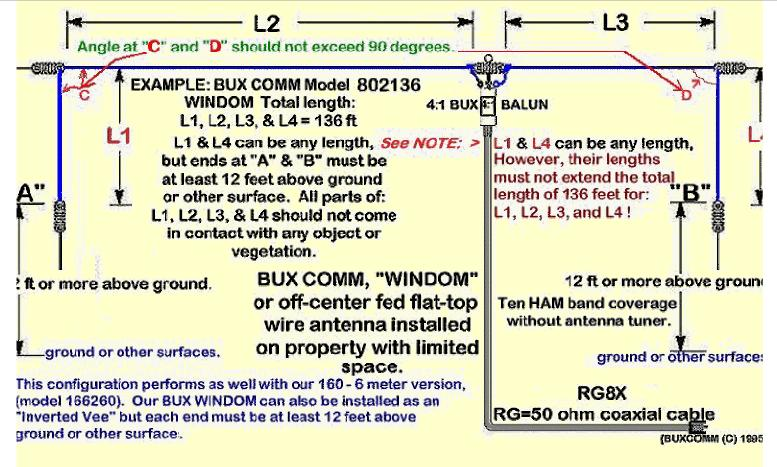
e Windom can be installed as a Droop-End (see figure D below) or as a sloper, but in no case, should the angle be later than 90 degrees against itself. To use an angle that folds against the pattern of the opposite end, or the feed line of Windom, could change the impedance of the feed-point, change the multi-band features, and most important, destroughted the contract of the antenna.
