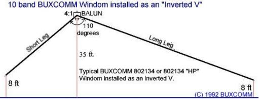
Windom total length is 134 ft, when installed as an Inverted V, distance required is 118 ft.
