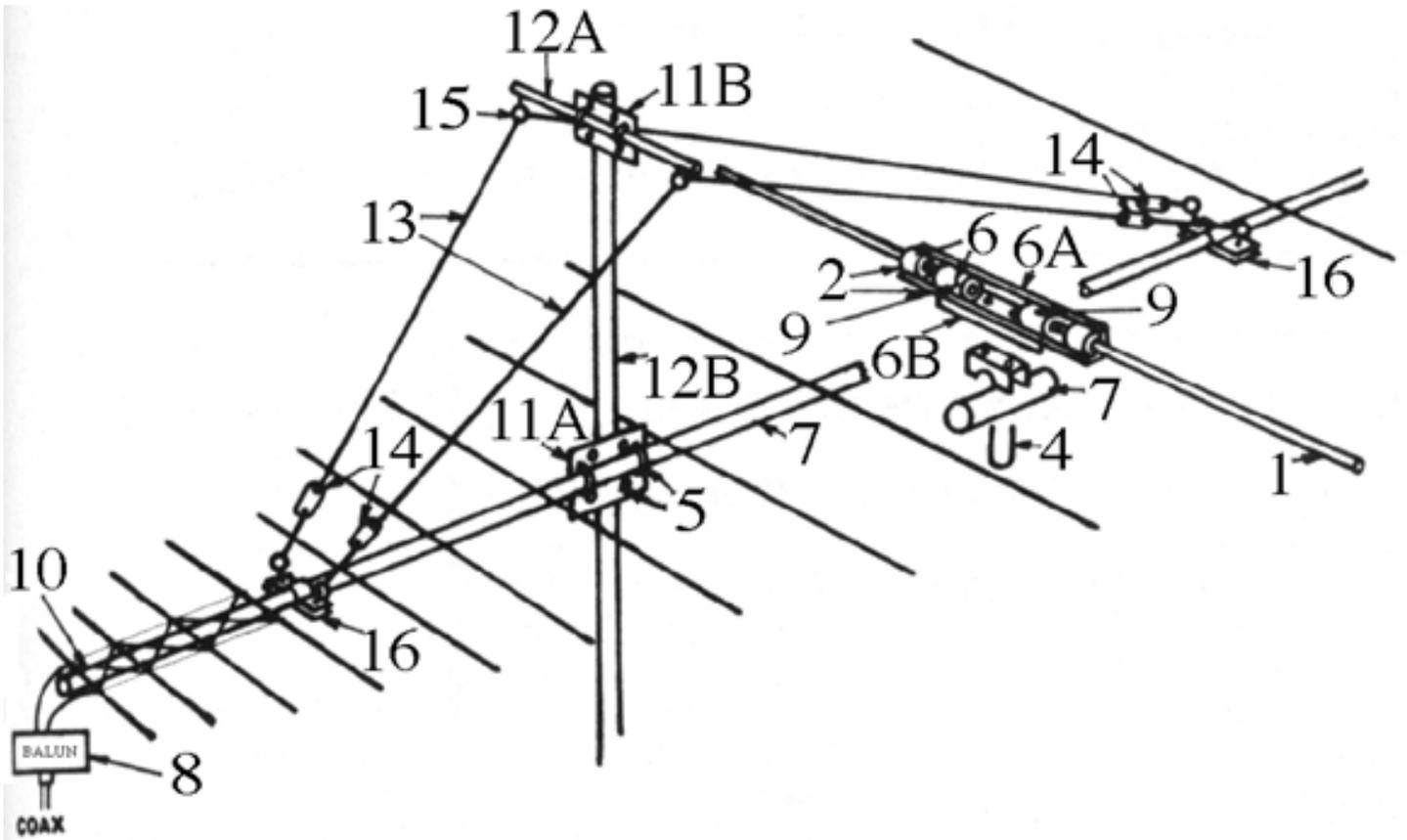
Fig. 8 - Construction diagram of log-periodic array. Figure 9 and 10 are shown the method of making electrical connection to each half element, and at D is shown how the boom sections are joined.
