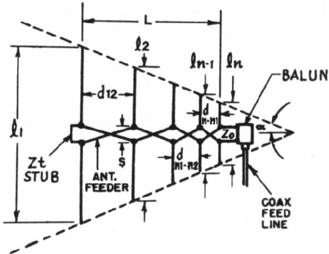
Fig. 1 - Schematic diagram of log-periodic dipole array, with some of the design parameters indicated. Design factors are:
