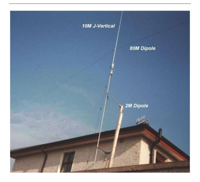
My first J vertical was a Slim Jim for two metres. This simple aerial performed better than a centre fed dipole at the same height. I compared it with an end fed half wave and an end fed 5/8 wave vertical. The Slim Jim always gave better results.
