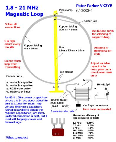
Magnetic loops are a compromise antenna and performance will be down on a full-size wire antenna, particularly on the lower HF bands. If built properly, expect the following results at QRP power levels: (i) 80 metres - contacts up to a few hundred kilometres, (ii) 40 & 30 metres - single hup contacts up to about 3000 kilometres with the occasional DX. The variable capacitor won't spark if transmit power is kept down (10w is fine).
