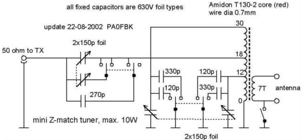
the Z-match principle has the big advantage that switching of the inductor is not necessary between the different bands,
