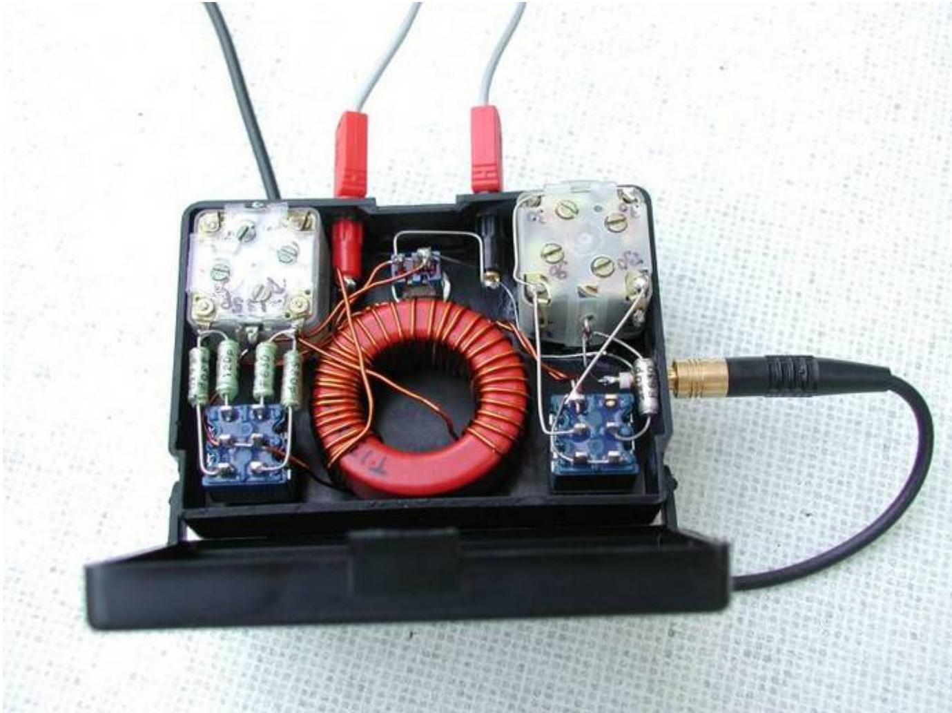
Inside the tuner, the 33mm Amidon core is the largest part. Notice the 630V fixed foil capacitors (four left, one right). Probably you can also use ceramic capacitors, mostly they have lower voltage rating, so try it out. The two antenna connectors are 2mm dia, the 50 ohm connector to the FT817 is an SMB type, coax is 3mm RG174. The 7 turns of the output winding must be wound at the ground part of the primary winding, as indicated in the diagram.
