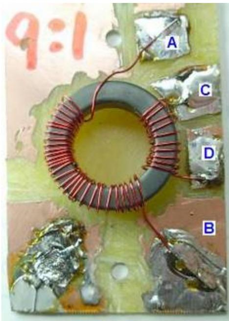
Next I tried a 9:1 impedance ratio UNUN. This an extremely popular impedance transformation ratio for end-fed or random wire SWL antennas. I wound 30 primary and 10 secondary turns on a FT114-43 ferrite toroid. The connection points are identical to those described in the above 4:1 UNUN. Remember that the impedance transformation ratio is the square of the actual turns ratio on your transformer; thus my 3:1 turns ratio is a 9:1 impedance ratio.
