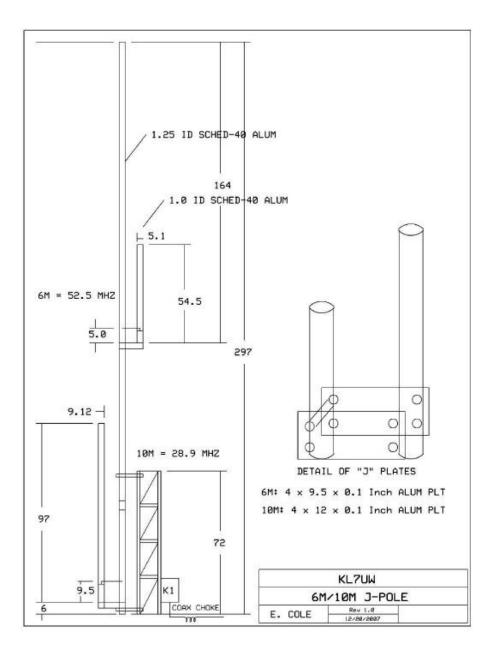
The antenna was initially designed using NEC4win95 antenna design software, but subsequently was taken from the excellent J-Pole calculator at <a href="DX-Zone">DX-Zone</a>. The calculator is for 1/2-inch copper tubing, but I substituted 1.25-inch schedule-40 aluminum tubing (1.66-inch O.D.). The tubing used in the "J" section are 1.0-inch aluminum tubing.
