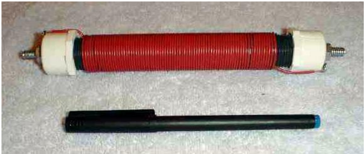
Figure 6: Photo of completed coil. (A pen is shown for size comparison.)
