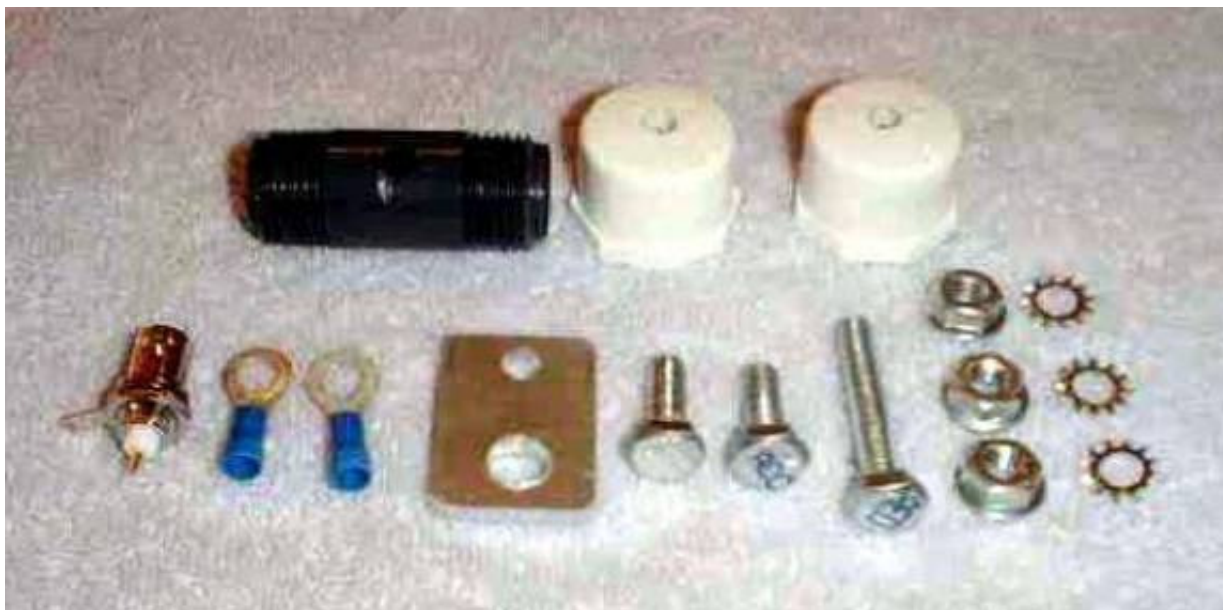
Figure 10A: Feedpoint insulator components
