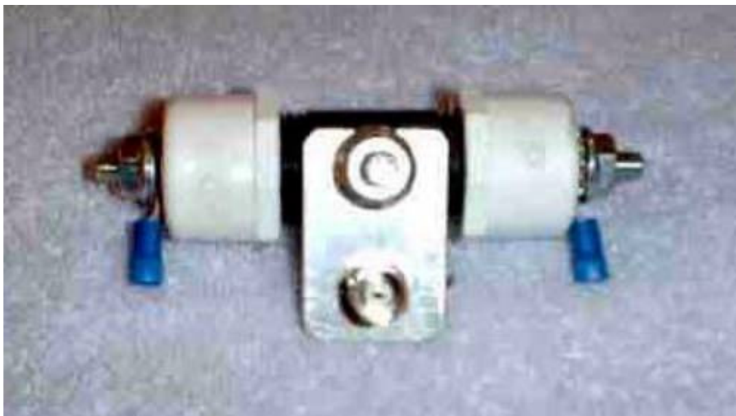
Figure 11: Completed feedpoint insulator
