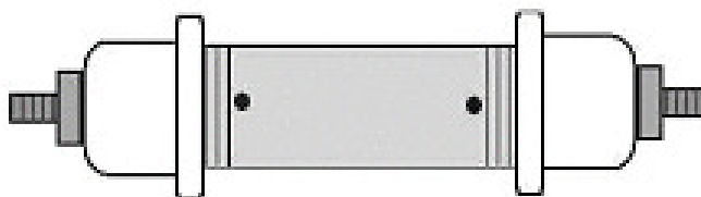
Figure 4: Completed coil form
