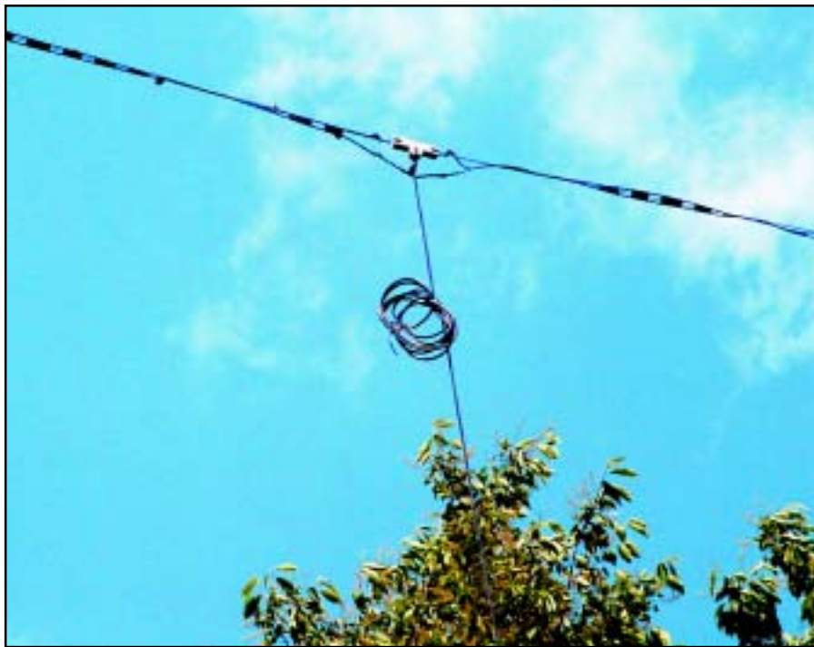
Figure 7— The K4VX 40-meter linear-loaded dipole deployed at 40 feet.
