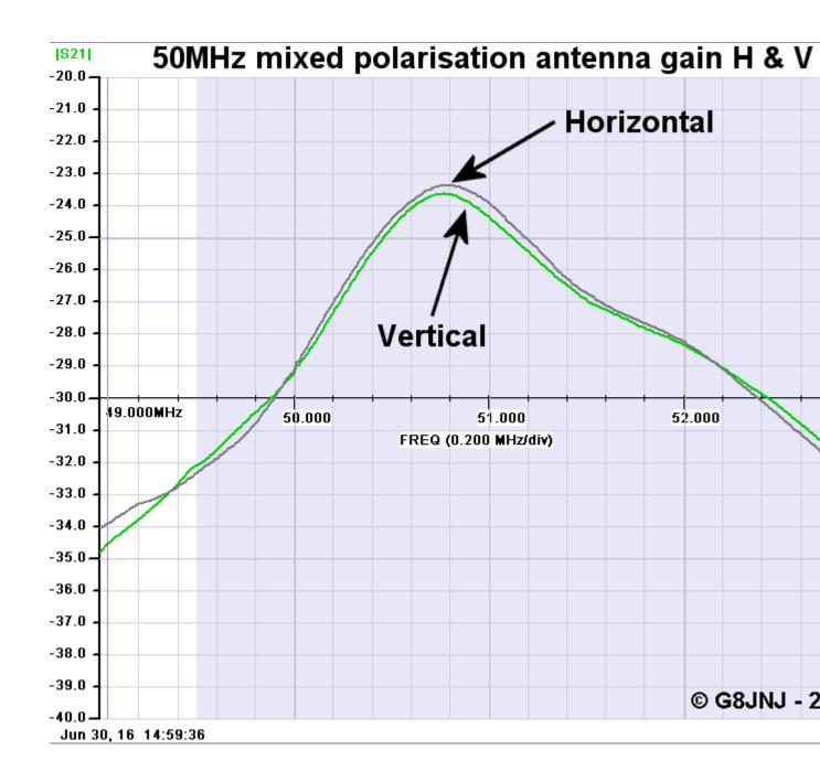
When using this antenna with JT65 on 6m, it produced about 30% more spots in the same 24 hour time frame, in comparison to a another receiver connected to a 1/4 wave vertical (V-2000) mounted at approximately the same height.
