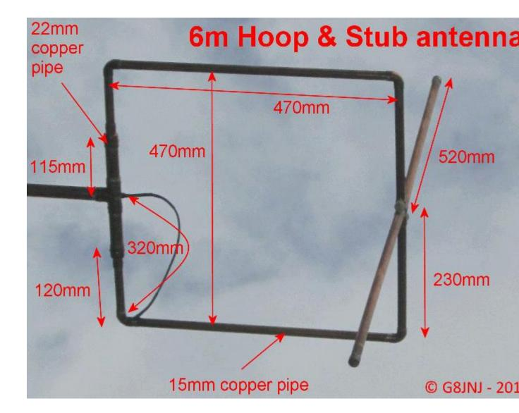
The antenna can be fine tuned by adjusting the thickness of the spacer between the two vertical sections.
