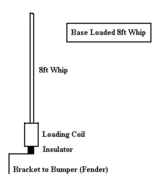
The base loading coil has to be mounted on a strong enough mount to take the normal flexing seen during mobile operation. Typically, the spring for the whip mount would be above the coil, allowing the whip to move without putting undue stress on the coil. Some commercial coils from the 50's had a bandswitch on coil allowing one to switch between the taps on the coil quickly.
