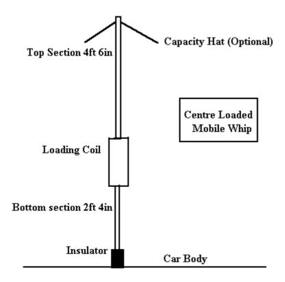
Typically, the bottom section is made of a larger diameter rigid section of tubing EMT, also known as conduit, makes a rugged makes a rugged bottom section, and the heavy galvanizing not only protects it from the elements, but allows one to solder directly to it for an improved connection. The zinc in the galvanized coating is a moderately good conductor, having a conductivity of 26 - 32% IACS. Copper, for comparison, has a conductivity of 100% IACS. Only silver is better.
