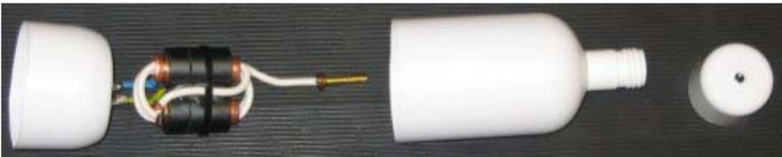
The top connector (in this case a 6mm brass bolt) is passed through the screw cap. This is tightened down before brass nuts and washers are placed on the bolt and fastened. This completes the assembly.
