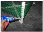
Winding the Coil on the PVC Frame The wire size and length recommendations in Table A have been tested in actual PVC loops, and should be followed for best results. In any case, wire should be stranded, insulated, single conductor, and of a size close to the wire recommended in Table A.
