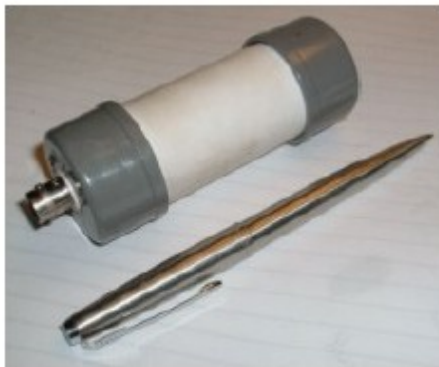
Fig. 5 De mini-whip in (witte) PVC-pijp
