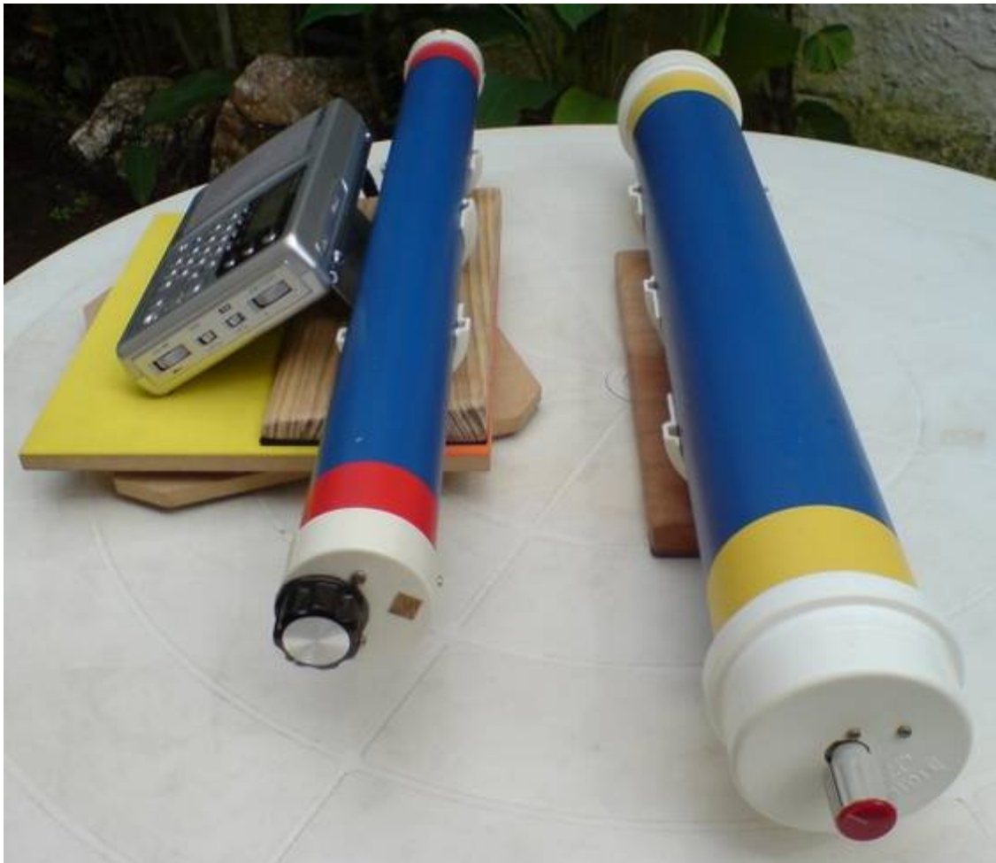
Comparing the 3 antennas, the original RGP3 and both extended loops, showed improvements only in the larger one
