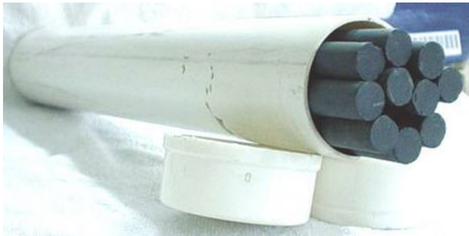
Using 40 mm pvc pipe cross section can accomodate 10 ferrite rods (10 mm diameter each)
