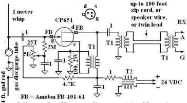
gas discharge tube = Xicon gas tube surge arrestor, Mouser # 444-GT-90L
