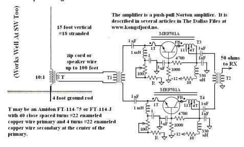
vertical was tested with twin lead up to 100 feet in length, so a pair of these separated by about 150 feet make a good MW phased array. If you are not a builder, you can buy an equivalent Norton amp from <u>Kiwa Electronics</u> for about \$110 plus shipping (as of October 2006).
