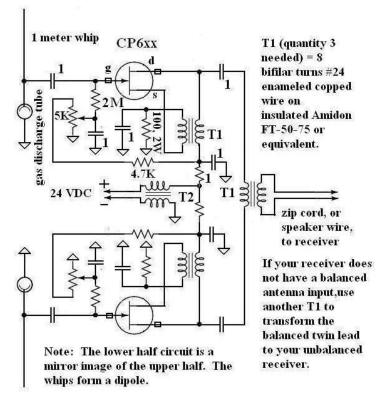
T2 (quantity 1 needed) = 30 bifilatr turns #22 enameled copper wire on insulated Amidon FT-114-75 or -J or equivalent.
