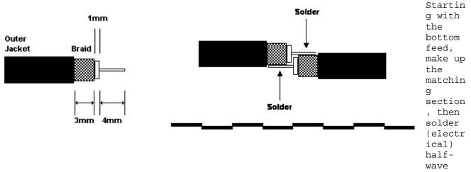
sections, alternating the center and shield for the ends. The image will better illustrate this method.
