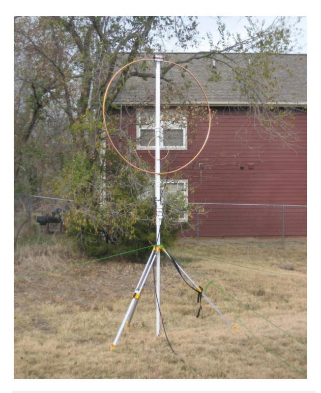
This loop was a little different than the others, in that I didn't try to use a single capacitor to tune it. Instead, it used two capacitors arranged in parallel. The first was a vacuum-fixed capacitor, 100pF, to provide most of the 120pF required to bring the resonant frequency down to around 7,500kHz. The second capacitor was a smaller 3-30pF vacuum-variable, used to provide the tuning adjustment to pull the frequency down further into the 40m band.
