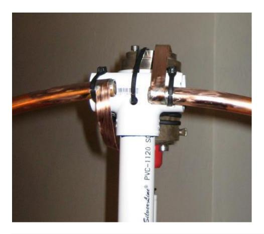
Note that the copper and solder around the joints was polished after assembly. This removed the discoloration and oxidation that naturally occurs when using a torch for soldering. Again, the skin effect of RF flowing on the surface of a conductor adds enough resistance on its own. I hoped the polish would make sure that the current wasn't flowing through any additional impurities.
