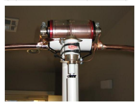
The initial tests of the 40m loop were very promising. During a CW contest, the 40m loop made numerous DX contacts in Europe. When running at 500W, the capacitors showed no signs of heating (SWR drift, physical warmth, etc.).
