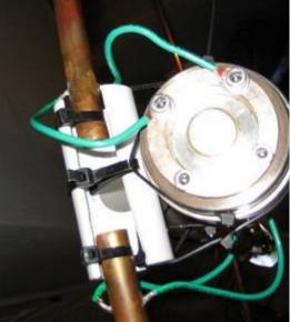
You will note that I used wires to connect the ends of the inductor to the capacitor. Although this wasn't optimal from the standpoint of keeping resistance low, the Q of the loop remained quite high after this change. More importantly, I could tune the loop to any frequency from 20m through the CW/data portion of 10m.
