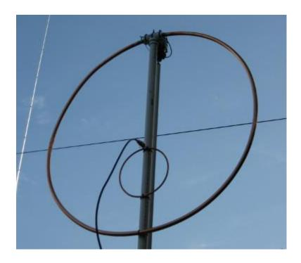
A few QSOs later, it was time to add a motor drive to the capacitor, so that I could remotely tune the loop.
