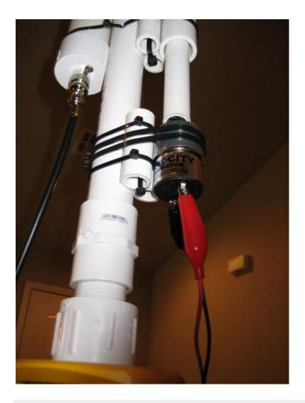
I added a couple of protection items to the motor before using it. First, I placed a 0.05uF capacitor across the motor's DC terminals. This keeps the RF out of the motor windings. Second, I choked the power leads with a common mode snap-on bead, to keep RF from flowing into the motor from the long leads, or back to the power supply from the motor. The motors also had a vinyl cover added, to weatherproof them.
