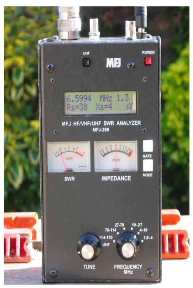
Now I'm on the 45 meter band. This brings back memories. Trial and error brought the resonant frequency into the 40 meter band at around 7.38 meters each leg. Try it - but careful when you start chopping the odd centimeter off the ends, each centimeter was worth about 50KHz in resonant frequency as I remember it.
