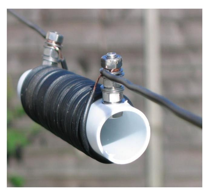
Close up of the coils under tension. The conclusion was that it worked really well and compared well to the (40 meter delta loop). Less than 1.3:1 SWR at 7.120 MHz with less than 3:1 SWR band edge from 7.04 MHz through to 7.2 MHz, the whole UK 40 (7 MHz band) meter band for five quid. Let me know how you get on.
