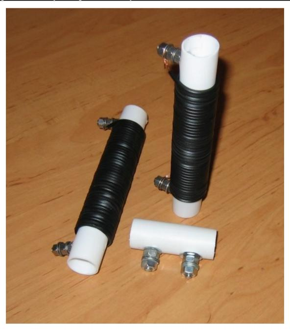
Here's some coils I made from plumbers pipe together with a dipole centre.
