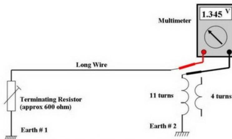
Figure 4: Earth Resistance Measurement
