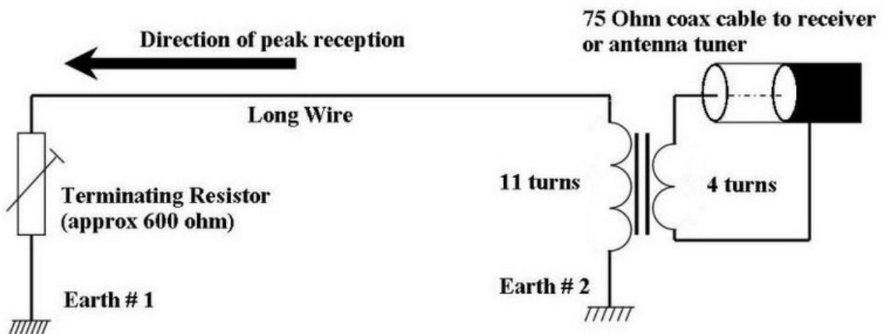
**Figure 1:** A basic uni-directional Beverage antenna
