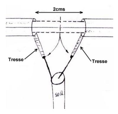
Although identifying the center of the coax, and remove the insulation on 2cms length Cut the braid in the center and fold the two pieces to the edge of the sheath.
