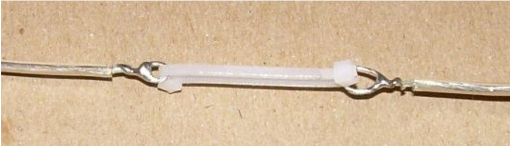
**Detail of soldered loops and 1.4" zip tie connection between driven and reflector elements**
